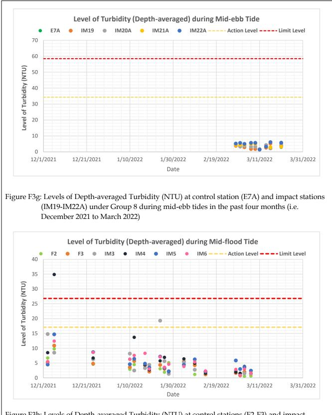
Figure F3h: Levels of Depth-averaged Turbidity (NTU) at control stations (F2-F3) and impact stations (IM3-IM6) under Group 2 during mid-flood tides in the past four months (i.e. December 2021 to March 2022)
