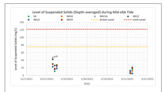
Figure F4c: Levels of Depth-averaged Suspended Solids (mg/L) at control station (E4) and impact stations (IM10-IM14) under Group 4 during mid-ebb tides in the past four months (i.e. December 2021 to March 2022)
