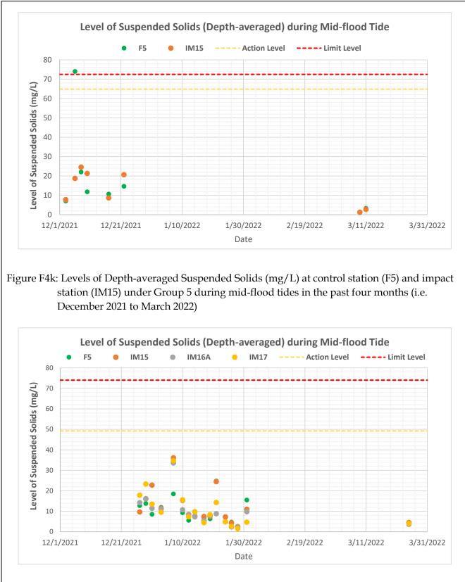
Figure F4I: Levels of Depth-averaged Suspended Solids (mg/L) at control station (F5) and impact stations (IM15-IM17) under Group 6 during mid-flood tides in the past four months (i.e. December 2021 to March 2022)
