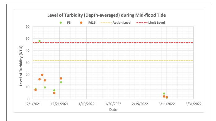
Figure F3k: Levels of Depth-averaged Turbidity (NTU) at control station (F5) and impact station (IM15) under Group 5 during mid-flood tides in the past four months (i.e. December 2021 to March 2022)
