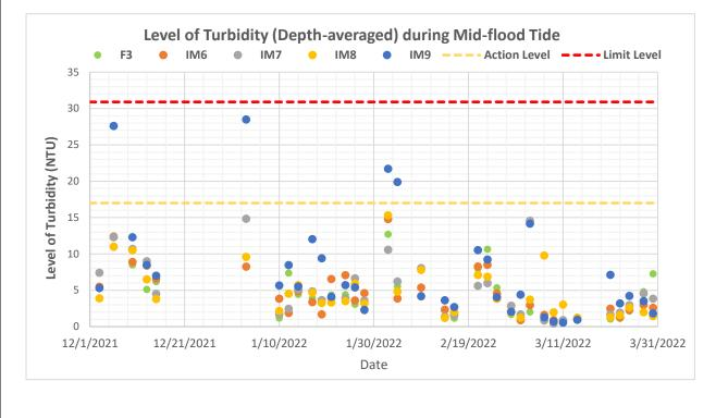
Figure F3i: Levels of Depth-averaged Turbidity (NTU) at control station (F3) and impact stations (IM6-IM9) under Group 3 during mid-flood tides in the past four months (i.e. December 2021 to March 2022)
