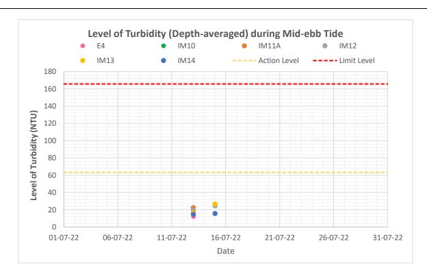
Figure F3a: Levels of Depth-averaged Turbidity (NTU) at control station (E4) and impact stations (IM10-IM14) under Group 4 during mid-ebb tides in July 2022.
