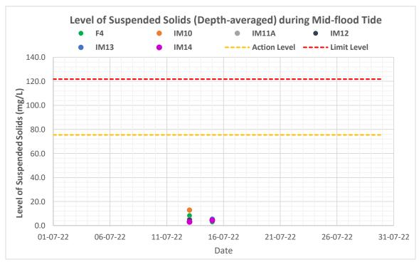
Figure F4b: Levels of Depth-averaged Suspended Solids (mg/L) at control station (F4) and impact stations (IM10-IM14) under Group 4 during mid-flood tides in July 2022.
