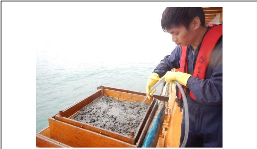
c) The sediment sample was sieved on site using a sieve stack.
