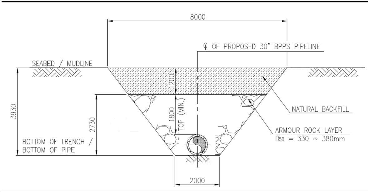
**Figure 2.6 Trench Design (Type F)**
