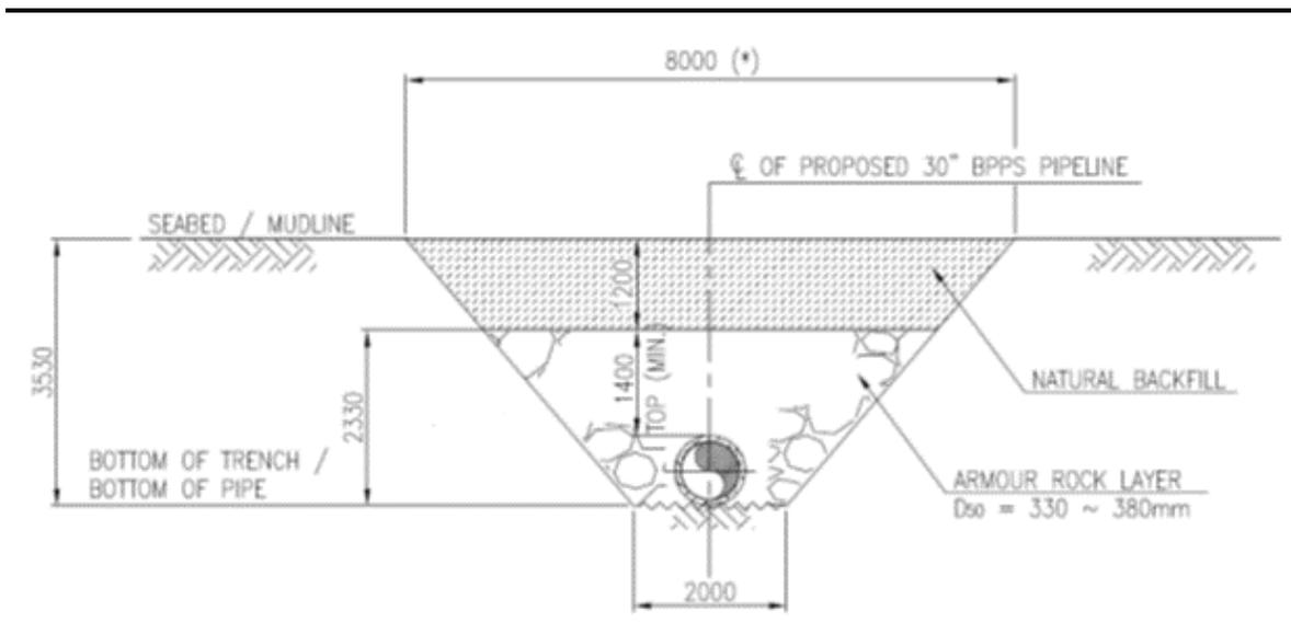
**Figure 2.5 Trench Design (Type E)**
