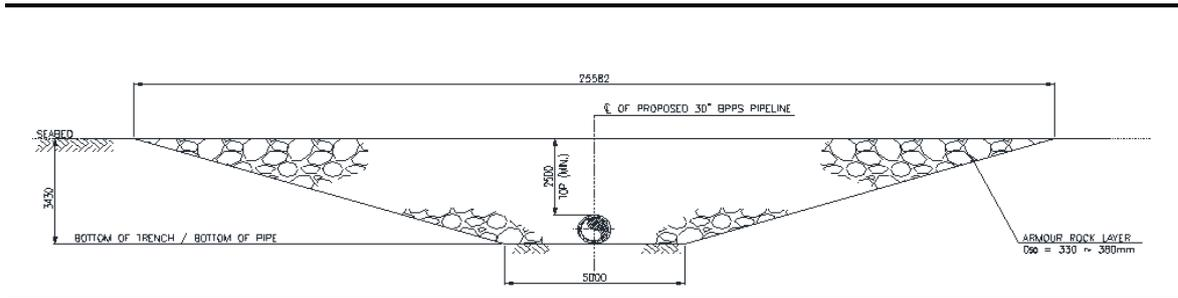
**Figure 2.7 Trench Design (Type G)**
